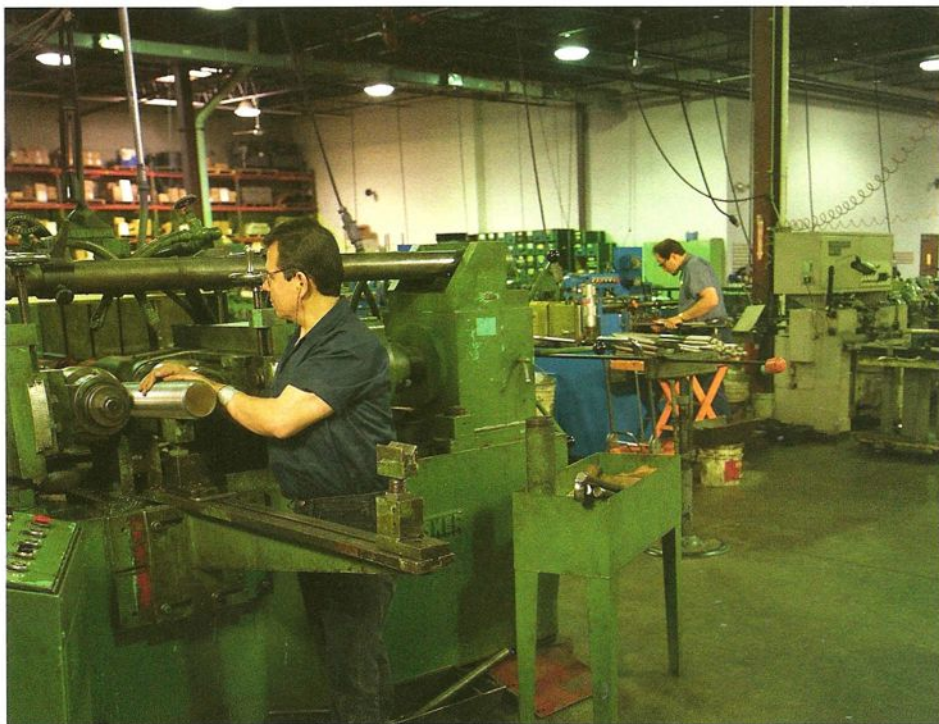
Tuttle Manufacturing can roll up to 6" diameter threaded rod or studs.
