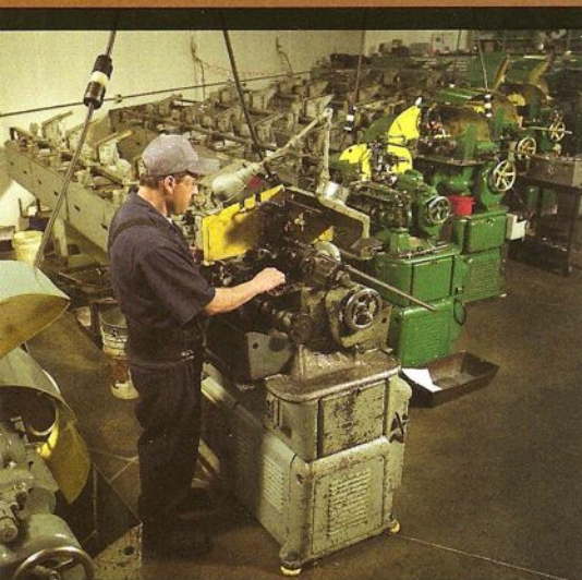
Partial view of a bank of Brown & Sharpe screw machines.
